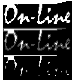
Figure 8: Original image (above) with the corresponding eroded one (below). In the middle, gray pixels would be the eliminated pixels in a voxel-oriented approach
